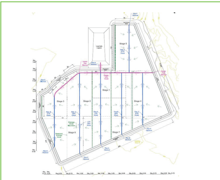
Figure 3 - An external lined leachate lagoon at a lower elevation allows leachate to continuously flow without periodic flooding and surging in the LCS which exacerbates clogging. Stage 1 was built first and the subsequent cells will connect and gravity drain through stage 1 to the lagoon.
