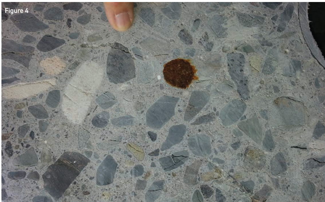
Figure 4. Cross-section of bridge barrier suffering from ASR and freeze-thaw deterioration.
