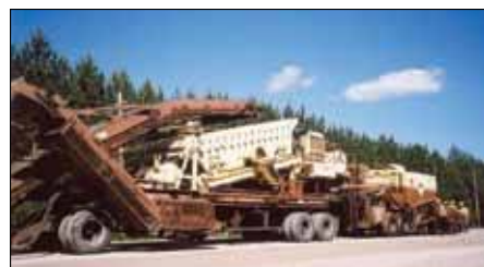
FIGURE 2A: Cold In-place Recycling (CIR) train (Chan et al. 2009).
