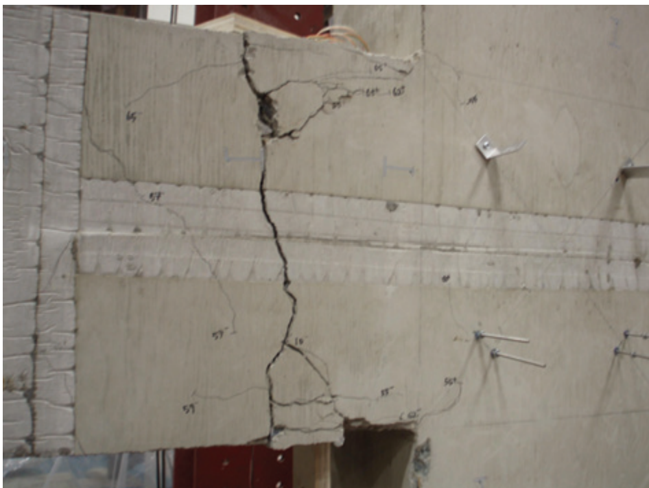
Figure 3(a): SMA beam-column joint (Youssef et al. 2008).
