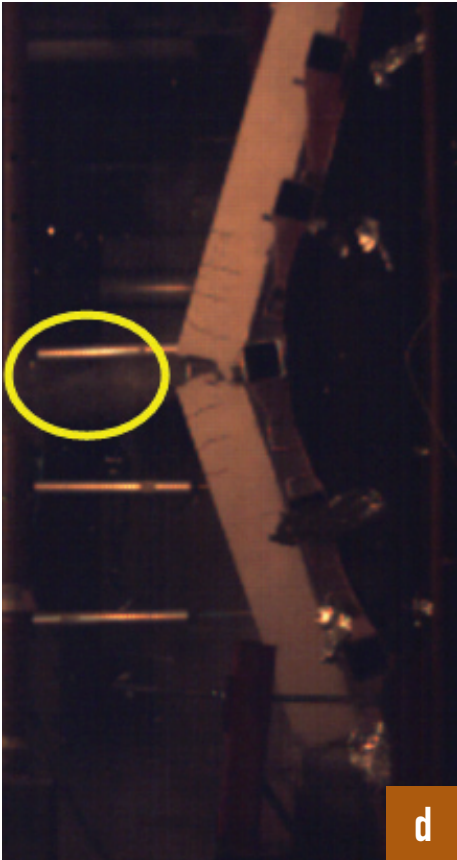
Figure 4: High-speed video stills of columns under blast loading: (a) SCC-0%-75 - Blast 3; (b) SCC-1.5%-75 - Blast 3; (c) CRC-2%-75 - Blast 3; (d) CRC-2%-75 - Blast 4 (Burrell et al. 2013a, b).
