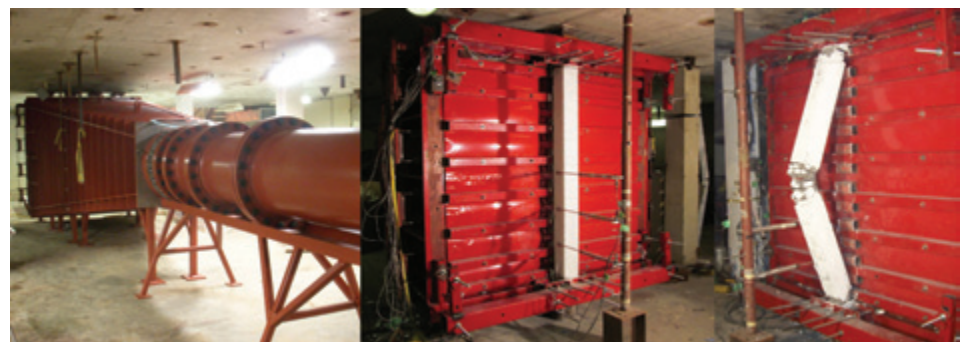
Figure 1: Blast testing of columns: University of Ottawa shock tube (left), column test setup (centre), and typical column after testing (right).
