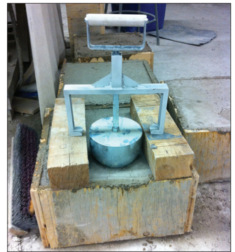
FIGURE 3: Ball drop apparatus.
