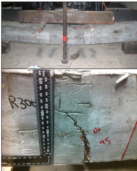
FIGURE 4: Test set-up showing typical failure of full cast slab-beam specimens.
