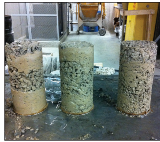
FIGURE 5: U-Fill samples produced from crushed granular at variable water contents: 210 kg/m 3 (left), 185 kg/m 3 (center) and 165 kg/m 3 (right).
