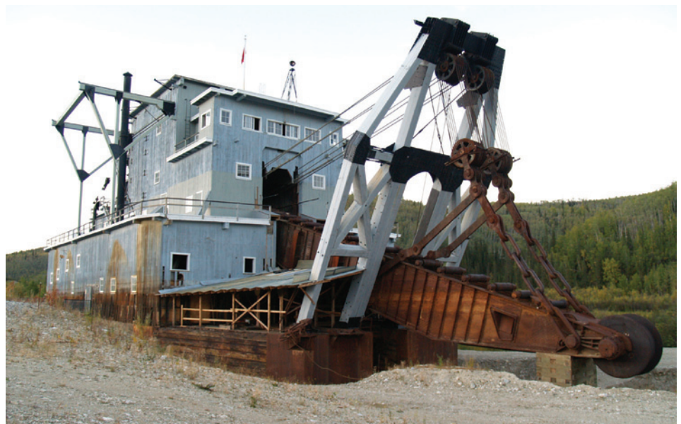
The massive, eight-storey Dredge No. 4 searched for gold on the Klondike River in 1913.
