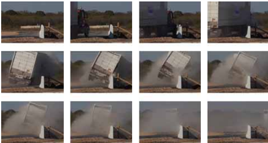
FIGURE 14: Sequential Photographs for the Crash Test (frontal views).
