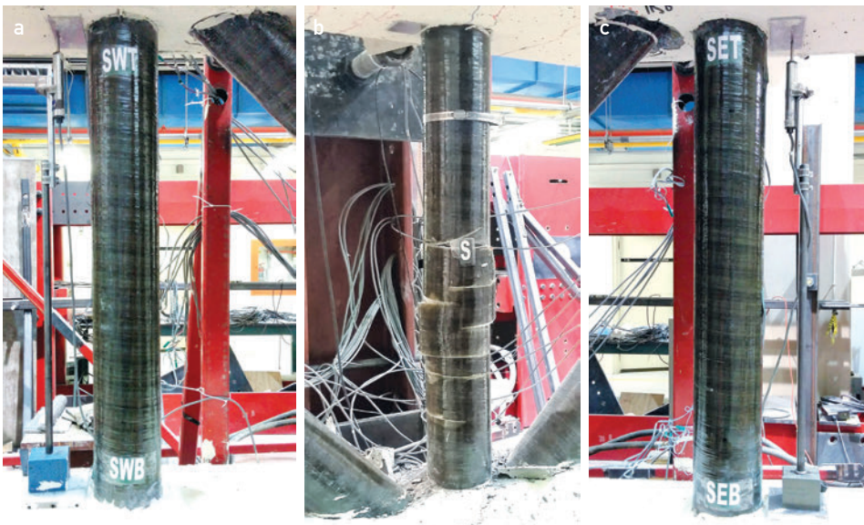
Figure 5: Vertical truss elements of Girder 1 at the end of test: (a) west element; (b) rupture of GFRP tube of central element; (c) east element
