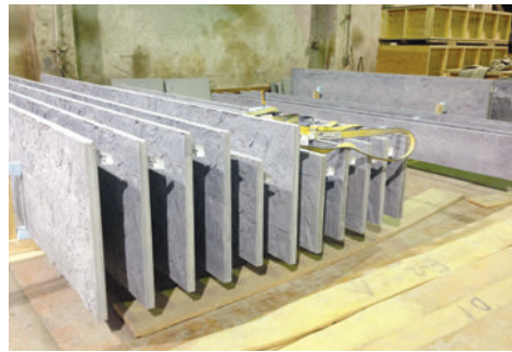
Top left: Fly-by corners. Above: The building façade combines glass, metal, and UHPC panels. Far left: Panel texture resembles stone in appearance. Left: Assortment of UHPC panels after casting.
