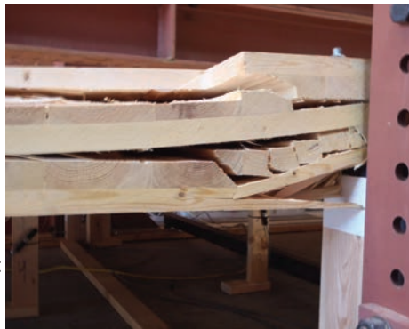
Figure 3: Point supported CLT panel testing apparatus and failure.
