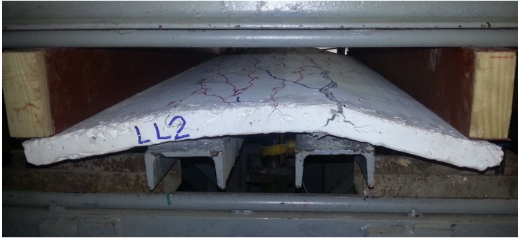
Figure 12 Slab Deflection and Mesh Failure at Ultimate Line Load
