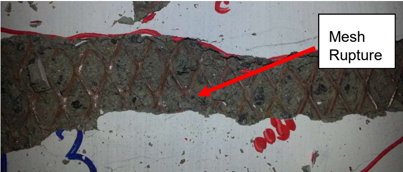
Figure 11 Crack Patterns Under Line Loading
