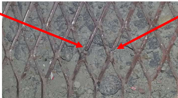
Figure 13 Crack Patterns Under Uniform Load
