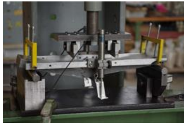
Figure 3: Four-point bending set-up according to the French code (Dobrusky, 2017)
