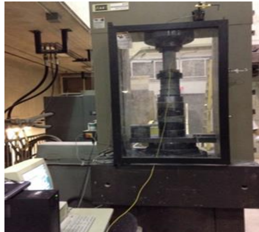
Figure 1: Cylinders equipped with FBG sensors (left) and the MTS machine used for testing (right) (Othman & Marzouk, 2016)
