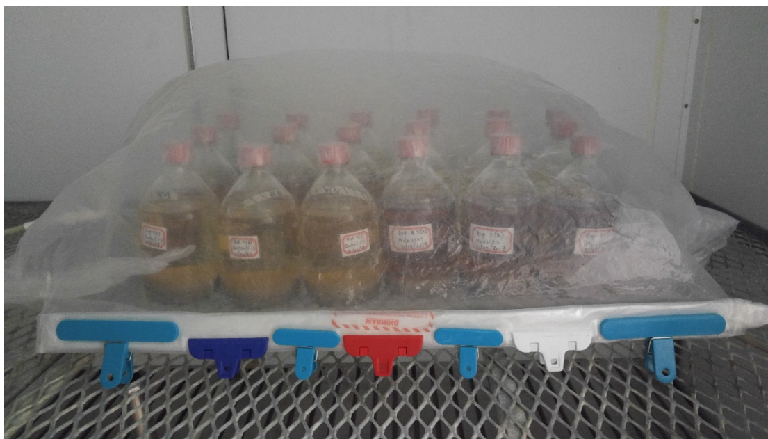
Figure 2: An example experimental anaerobic bag chamber shown in the controlled temperature chamber in the Phytotron facility of the University of Saskatchewan
