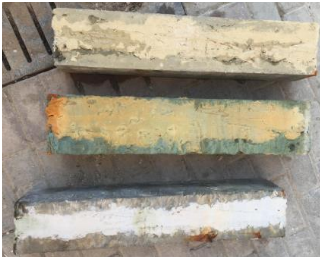
Figure 6 - Showing the effect of chemicals on the specimens, Fresh water effect (Top Beam), Magnesium Sulphate (Middle Beam) and Brine Water Effect (Bottom Beam)
