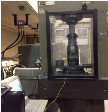
Figure 3 Compressive Strength and Modulus of elasticity test with embedded FBG sensor (Yazidizadeh 2014).
