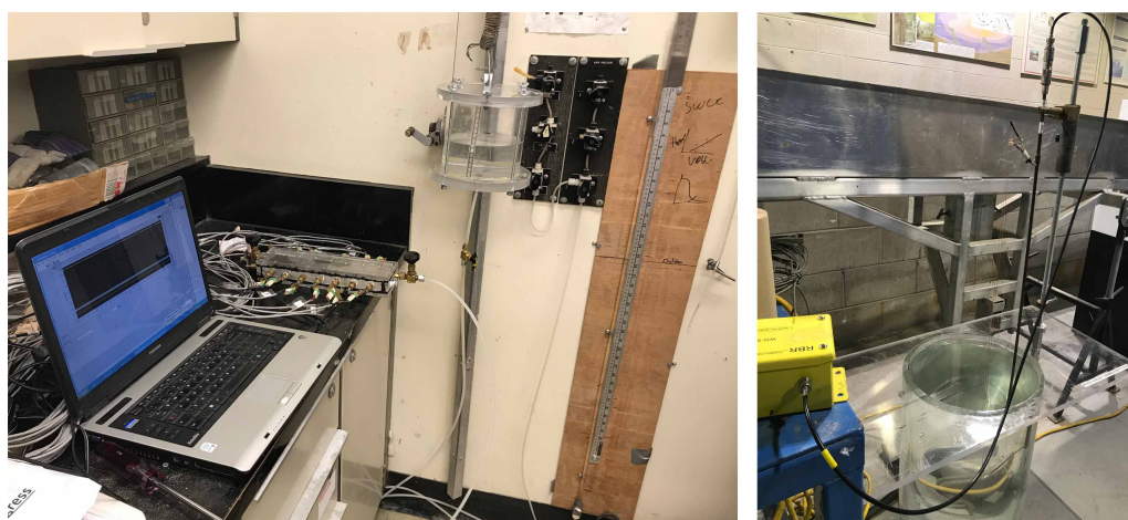
Figure 3: Calibration Process: left photo - tensiometers; right photo - wave gauges
