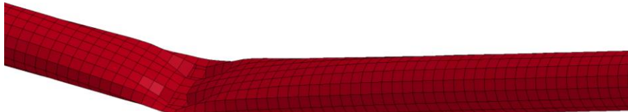
Figure 6: Local buckling failure of the pole in the finite element analysis
