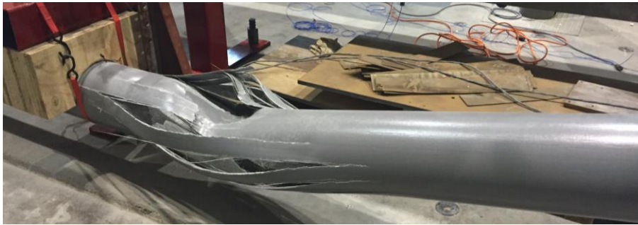
Figure 5: Local buckling failure of the tested pole
