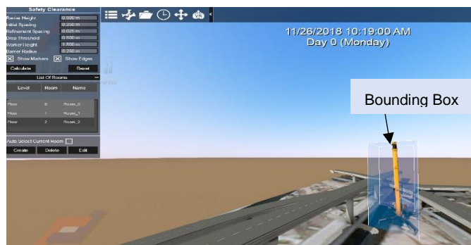
Figure 5: Bounding box for equipment workspace
