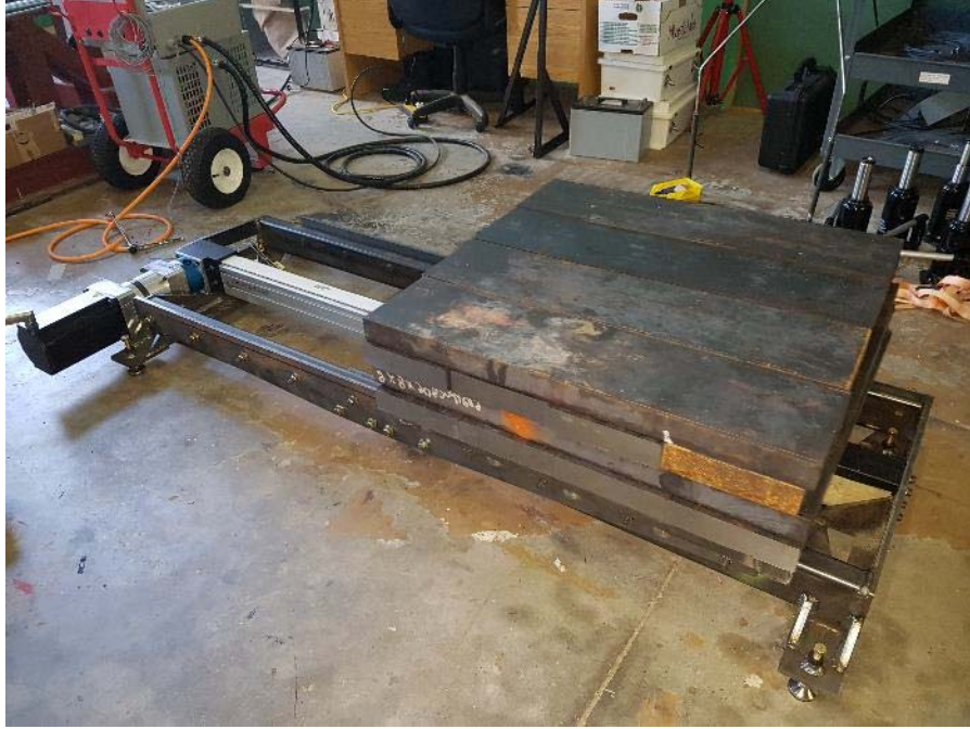
Figure 2: Building Oscillator with 1-ton mass developed by Gradient Wind Engineering Inc.
