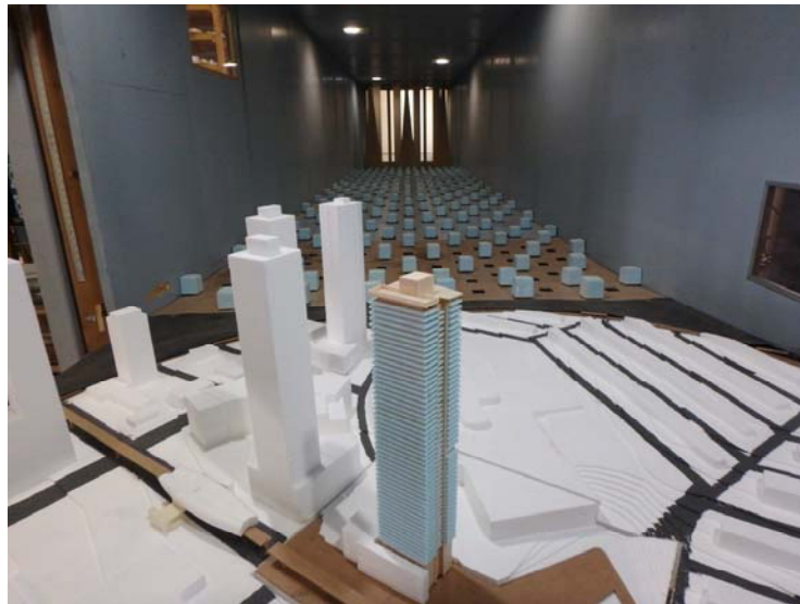
Figure 3: High-Frequency Force Balance (HFFB) wind tunnel testing of study building - Gradient Wind Engineering Inc.
