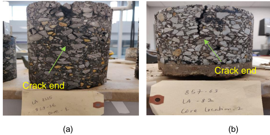
Figure 6: Cores showing longitudinal top-down cracks for control sections (a) 829-26 (b) 857-63
