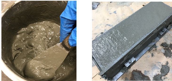
Figure 2: Preparation and Casting of PVA-ECC
