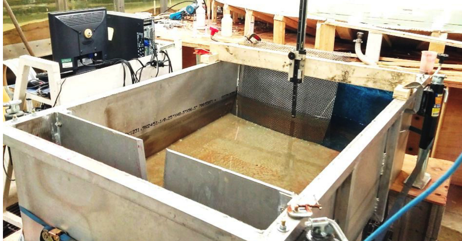
Figure 2: Weir box for the measuring the flow rate through the outlet of the model
