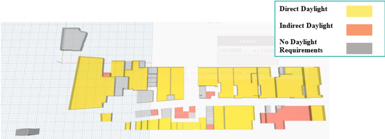
Figure 5 First Floor Daylight Requirements Compliance Assessment Visualization
