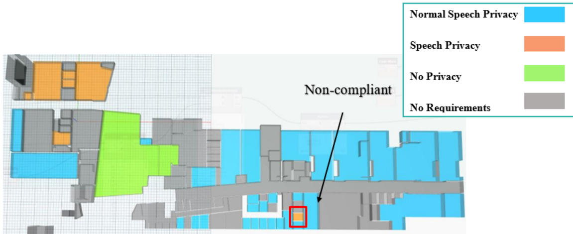
Figure 7 First Floor Acoustics Requirements Compliance Assessment Visualization
