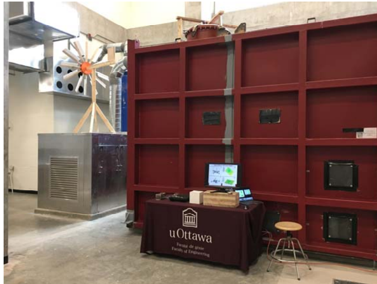
Figure 2: The Wind induced Damage Simulator (WDS)
