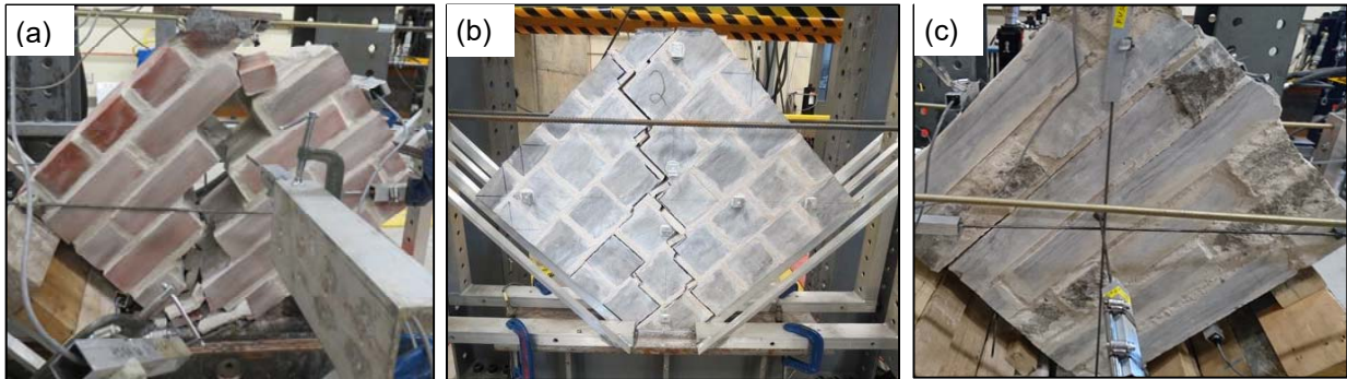
Figure 7: Diagonal tension failure of panels: (a) Brick panel A, (b) Sawn stone cubes, and (c) Guillotine stone blocks
