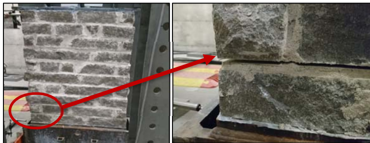
Figure 8: Rocking failure rupture of stone wallets
