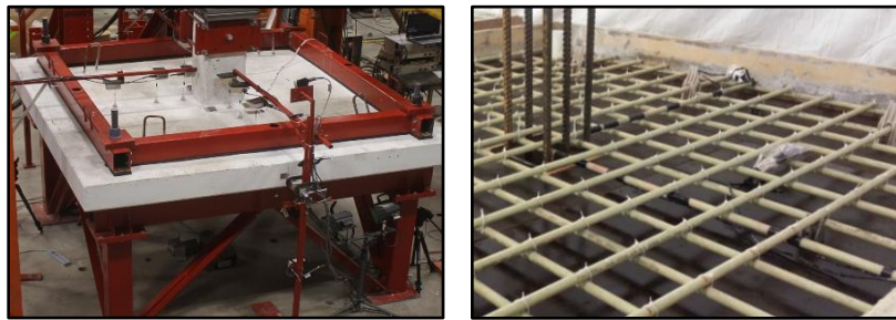
Figure 2: Position of internal and external instrumentations.
