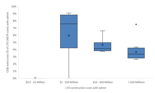
Figure 5: Widen Freeway-total CE&I costs as a percentage of the total LTD construction costs
