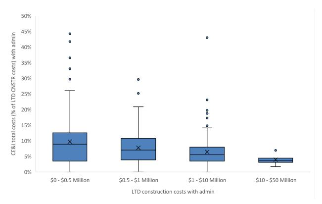
Figure 4: Bridge Replacement—total CE&I costs as a percentage of the total LTD construction costs
