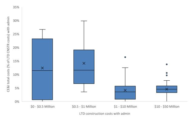
Figure 6. Widen Non-Freeway-total CE&I costs as a percentage of the total LTD construction costs
