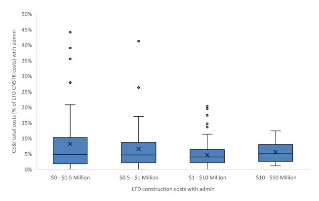
Figure 3: Miscellaneous Construction—total CE&I costs as a percentage of the total LTD construction costs
