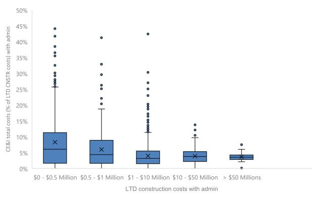
Figure 2: Total CE&I costs (% of total construction cost) versus project size
