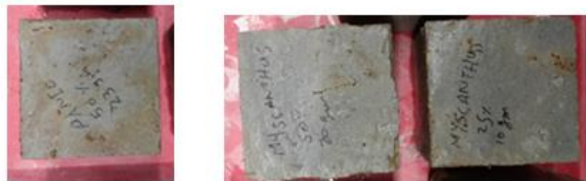
Figure 7 Expansion for samples with cement-based binder and agro-waste a) Piank and b) Myscanyhus
