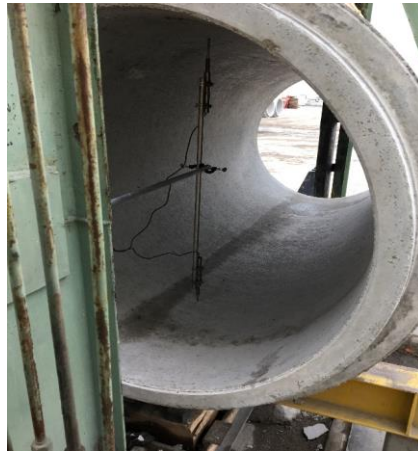
Figure 1: Setup of LVIT's when testing vertical deflection under TEBT
