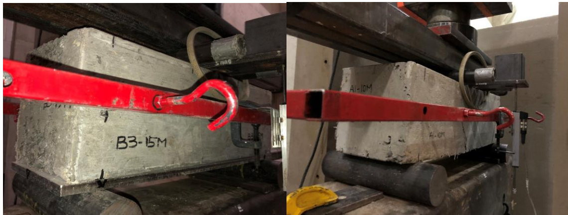
Figure 3: ASTM C1399 test setup (1.5% fiber)
