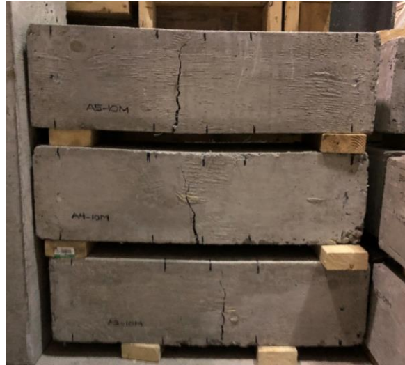
Figure 5: Tested FRC beams (ASTM C1609 - 1.0% fiber)
