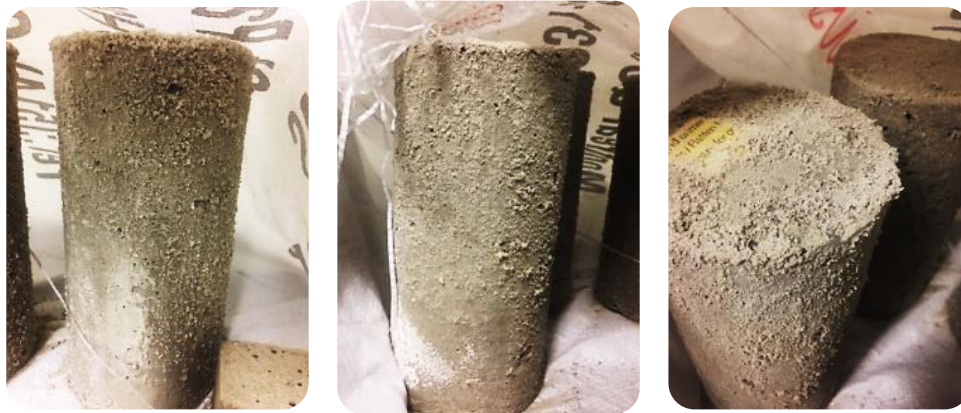
Figure 4: Efflorescence problem appeared in AASCC mixtures
