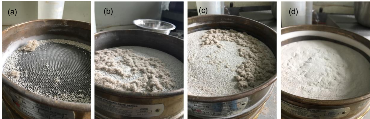
Figure 2. Gypsum retained of sieves (a) No. 16 (b) No. 30 (c) No. 50 (d) No. 100
