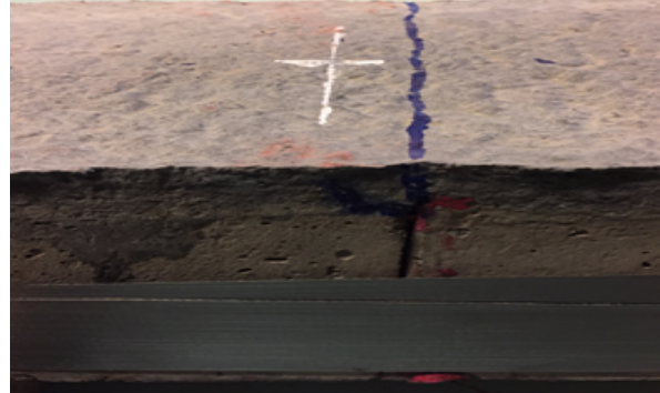
Figure 11: Unbonded Sample after 15,000 Cycles
