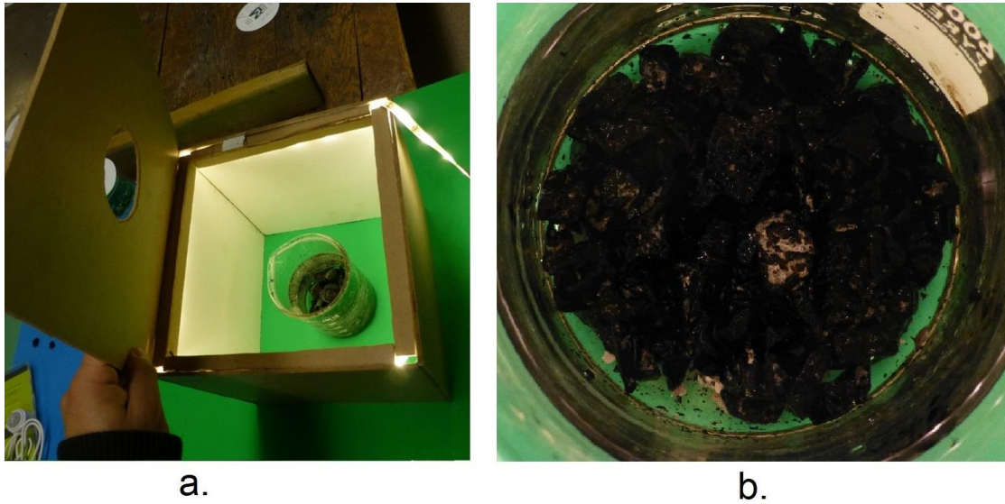
Figure 4. a) a lightbox prototype; b) sample image captured using this lightbox
