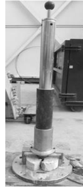
Figure 3: Impact test setup (Branston et al. 2016b)
