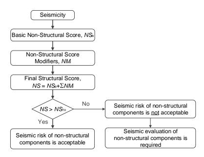
Figure 2: Non-structural scoring of existing buildings
