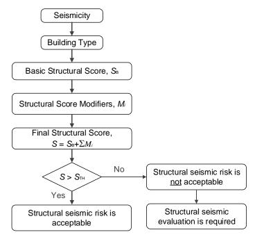
Figure 1: Structural scoring of existing buildings
