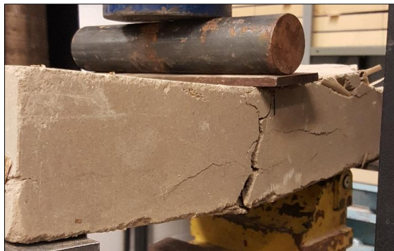
a) Flexural cracks after being loaded to failure
