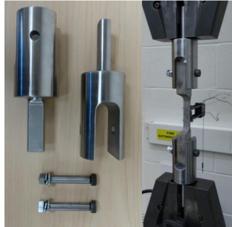
Figure 2: Testing of corner coupons with special grips and pins
