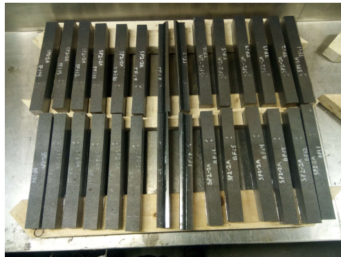
Figure 3: Flanges from specimen SP2-2A following sectioning
