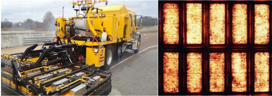
Figure 2: Left: Infrared Heating Machine in Use; Right: Bottom of Machine in Use (Kieswetter 2013)
