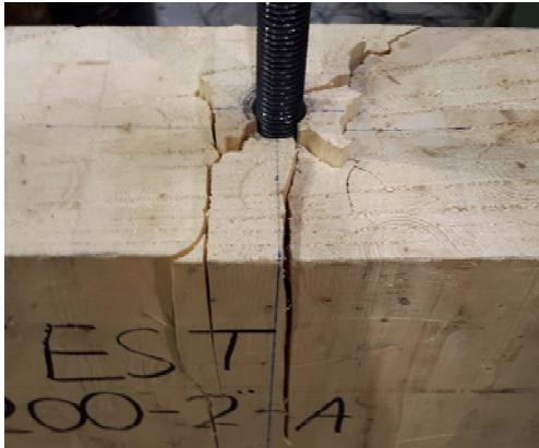
(a) Rod pull-out shearing along carved out hole with 45-degree cracks and beam splitting
