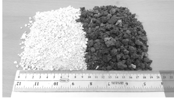
Figure 5: Lightweight coarse aggregate used Cicolite (right) and EP (left).
