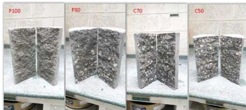
Figure 11: Some samples after splitting test.
