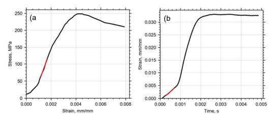
Figure 4: Determination of (a) Young's modulus and (b) strain rate
