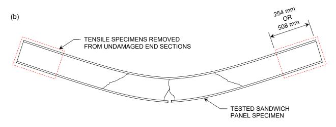
Figure 5: Specimen extraction: (a) sandwich panel and; (b) location of tensile specimen removal from sandwich panels tested by Betts et al. (2017)
