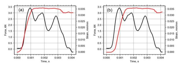
Figure 3: Load and strain data for specimen HR-AI-1 (a) as measured and (b) adjusted for time lag between measurements
