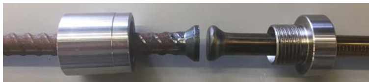
Figure 3. Mechanical couplers with headed deformed steel bar and headed SMA bar.
