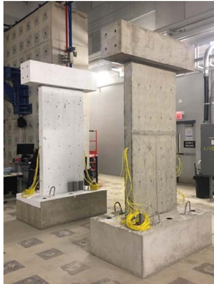
Figure 2. Walls after casting: SW-S (behind), SW-N (forward).
