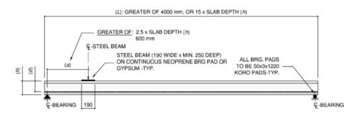
Figure 2 - Elevation of Typical Test Set-Up for Full Scale Shear Test
