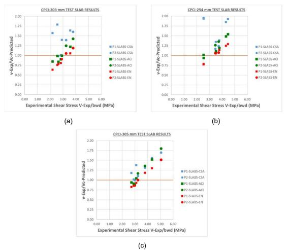
Figure 4 – Experimental versus Code Predicted Shear Capacity as a Function of Experimental Shear Stress, (a) 203 mm slabs, (b), 254 mm slabs, (c) 305 mm slabs
