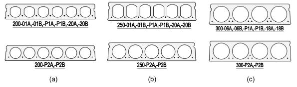
Figure 1 - Test Slab Identification (a) 204-mm slabs, (b) 254-mm slabs, (c) 305-mm slabs Table 1: Slab Identification
