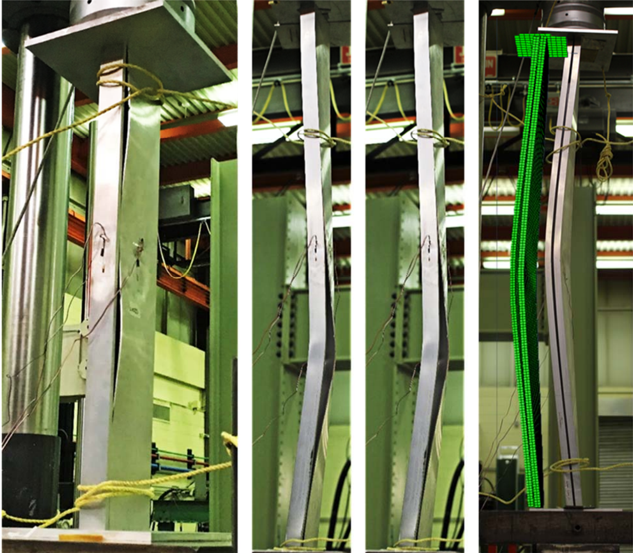
Figure 3: Test photos: (a) buckled Element 1, at 30% of ultimate load on 900 mm sample, (b) buckled 1800 mm sample (c) buckled 900 mm sample, and (d) buckled 1800 mm sample (with FEA model).
