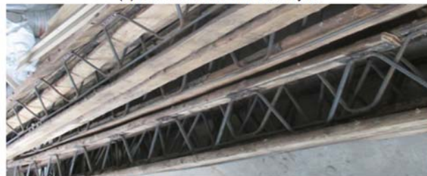
(b) A picture of the wood-steel joists
