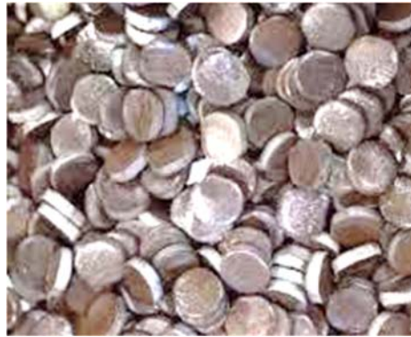
Figure 1: Steel chips used in this research as partial replacement of coarse aggregates
