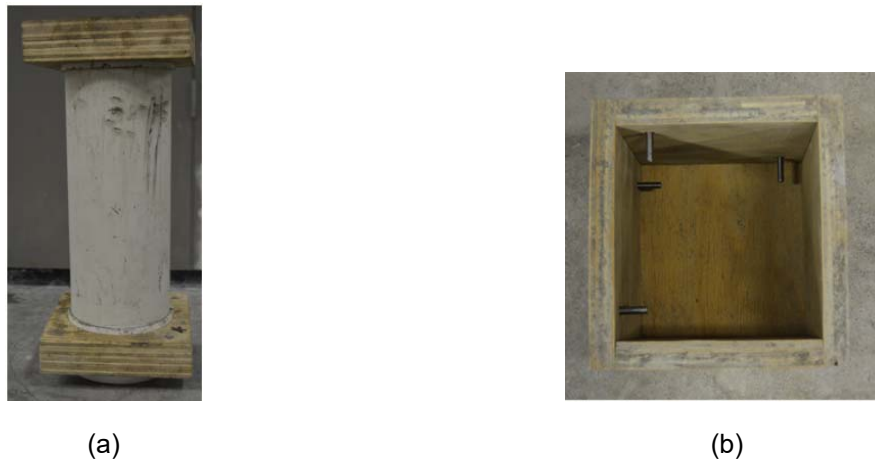
Figure 1: Molds for (a) cylinders and (b) cubes
