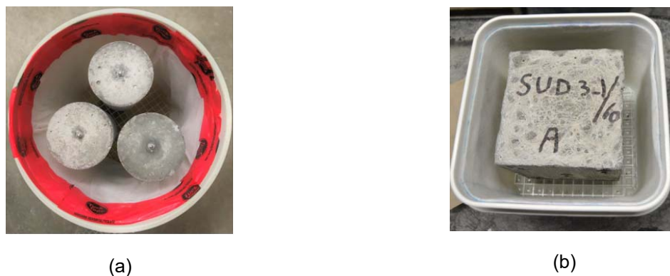
Figure 2: (a) Pails for the prism and cylinder samples (b) containers for cube samples
