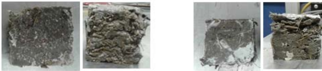
Figure 6 Expansion for samples with cement-based binder and agro waste a) Piank and b) Myscanyhus
