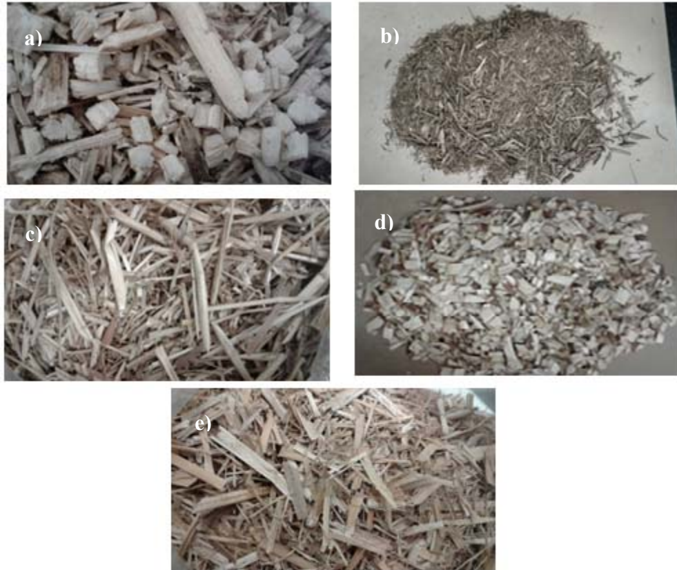
Figure 1: different agro waste samples, (a) Artichoke, (b) Spruce, (c) Savle, (d) Piank and (e) Myscanyhus.
